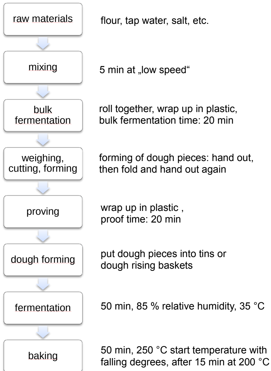
Fig. 5: Standard scheme for the manufacture of mixed rye-bread
