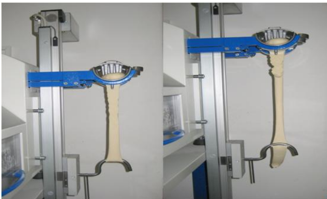
Fig. 4: Stretching the dough sample until rupture
