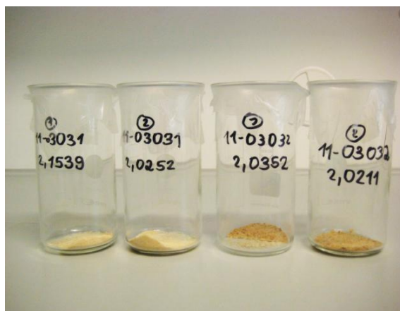
Fig. 11: Beakers with bread and roll samples, sealed with parafilm
