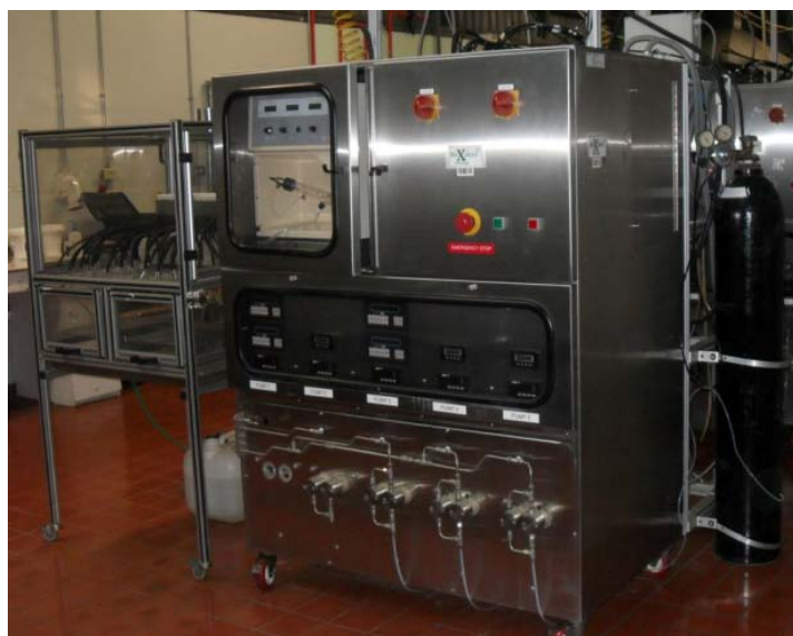
Figure 17: Industrial HPLC unit BioXplore 300, custom made by Varian.
