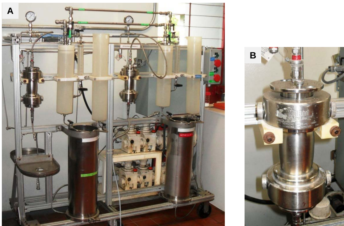
Figure 16: The charging station (A), equipped with a high-pressure column (B), was used for purification of crude extracts.
