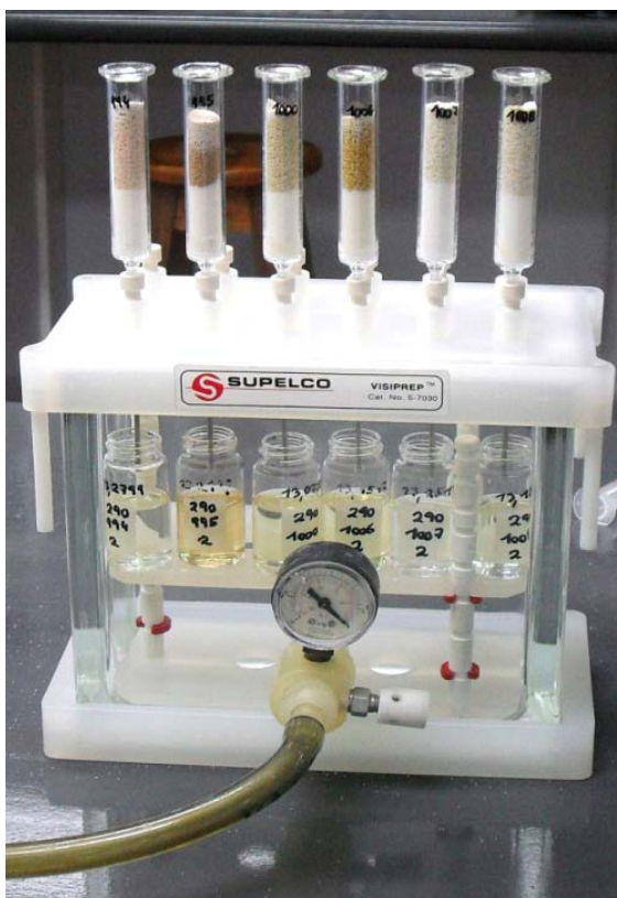
Figure 15: Supelco Visiprep™ SPE Vacuum Manifold, used for small-scale purification of the crude sponge extracts.
