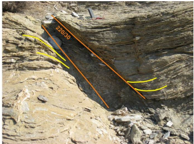
Fig. 34 (top): Normal drag along brittle/ductile high-angle faults. Outcrop number 22.
