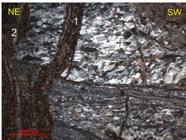
Fig. 92: Quartz-mylonite showing interaction of high- and low- angled fault development (xpl).
