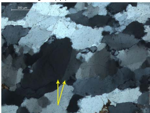
Fig. 66: Quartzite layer (within a carbonate schist); quartz shows undulose extinction, subgrain formation and grain boundary migration, yellow arrows point to two subgrains separated by a sharp subgrain boundary (xpl). Outcrop number 13.
