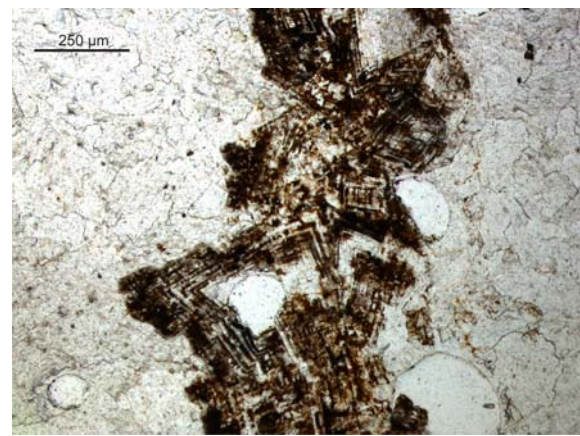
Fig. 80: Zoned ankeritic crystals in a calcite vein (ppl).
