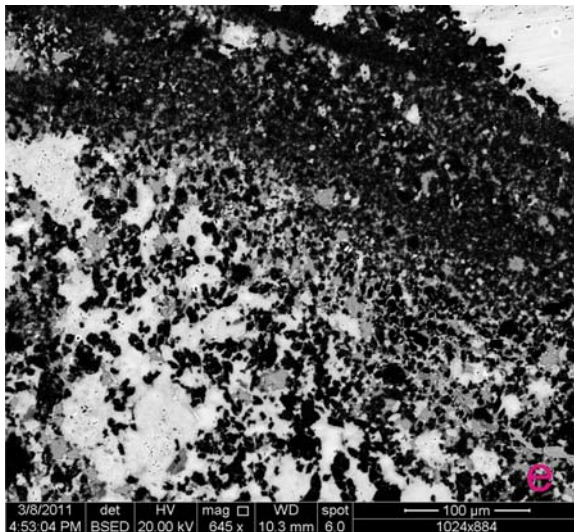
Smooth transitions between two ultracataclasites and a quartz vein.
