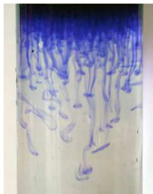
Figure 4: Saltfingers, [4] (priv. comm.), indoor experiment done with warm water and ink. The 'first generation fingers' can be observed.
