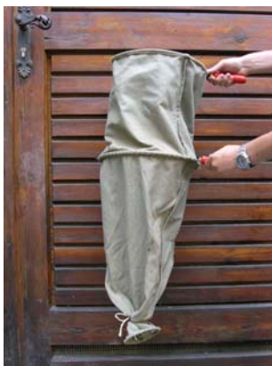
Fig.9. The use of a Reitter sifter for soil samples
