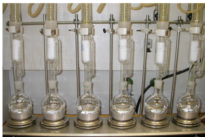
Fig. 18: Heatable extraction plant during Soxhlet extraction
