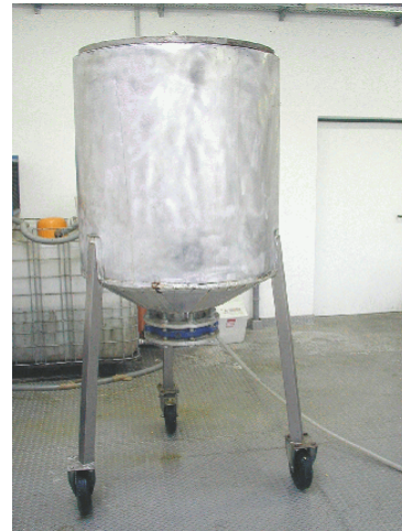
Fig. 9: Steep tank (ZFT, 2007)
